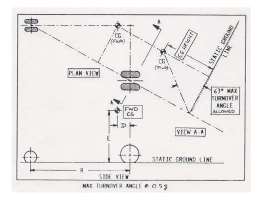
The height of the c.g. (E) is transferred to the scrap view (VIEW A-A) in order to calculate the turnover angle. The scrap view is a view as if looking parallel to a line on the ground which passes through the center of the MLG bogie and the nosewheel (this is the approximate axis about which the airplane will rotate if it were to tip over). The scrap view can be set at an arbitrary distance from the plan view so that it does not interfere with the plan view.
